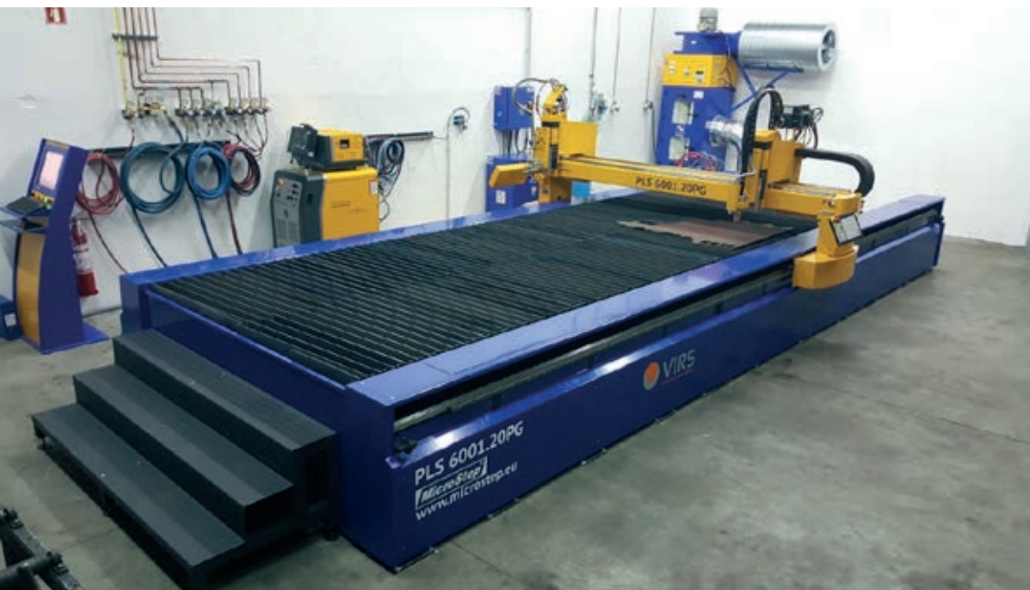
» Slika 6: Microstep PLS (plasma speed) hiter in dinamičen CNC-rezalnik s Kjellberg HiFocus 161i plazemskim izvorom
