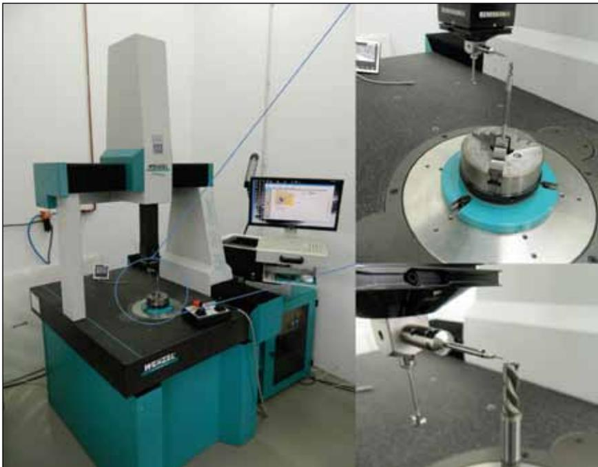
**Figure 16.** Coordinate measuring machine (CMM) Wenzel Gear Tec
