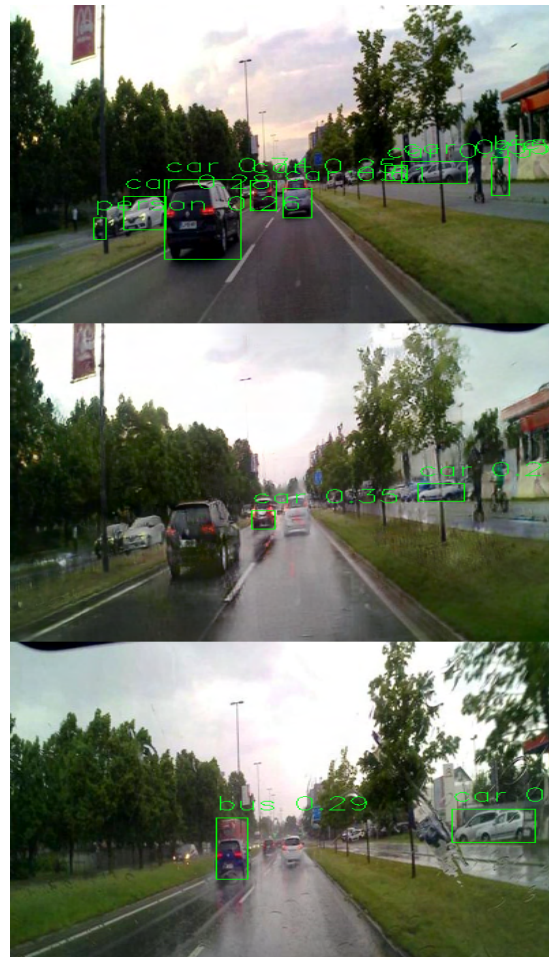
Figure 1: Successful style transfer mimicking real rain’s impact on vehicle detection. Top: input image; middle: simulated rainy image; bottom: style reference (rainy weather). Vehicle detection using YOLOv8 [11] shows significant performance drop from top (clear) to middle (rainy) image.
