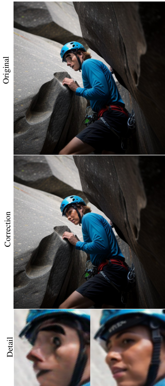
Figure 6: Example of the application of our method. Original image (top) contains severe artifacts in the facial area. Artifacts are discovered using our pre-trained classifier and multiple candidates for replacement are generated using inpainting. The candidates are again evaluated by our classifier and ranked according to its response. The one with the best score is selected as the replacement. The corrected images are shown in the middle row, while the details of the faces are depicted in the bottom row.
