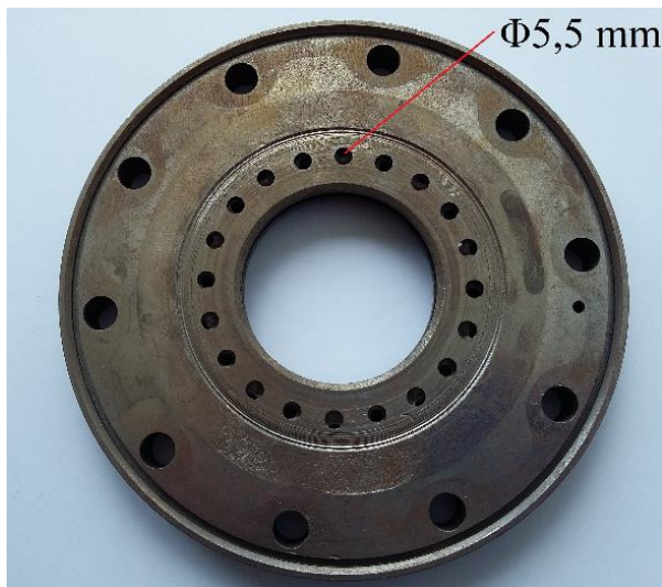
Figure 77: The minimal hole size (Φ5,5 mm) in the valve plate (Φ174 mm × 15 mm)
