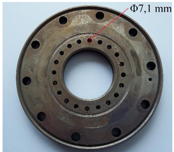
Figure 78: The desired maximal hole size (Φ7,1 mm) in the valve plate (Φ174 mm × 15 mm)
