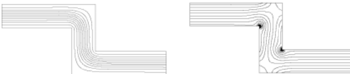
Sl. 9. Tok nenewtonske viskoelastične tekočine v kanalu oblike Z modelirane z zgornje konvektivnim Maxwellovim reološkim modelom ( \lambda_1=0,06 ); tokovnice (levo) in izošte vrtinčnosti (desno) Fig. 9. Non-Newtonian viscoelastic fluid flow in Z channel. Upper-convected Maxwell rheological model with ( \lambda_1=0.06 ); streamlines (left) and vorticity lines (right)
