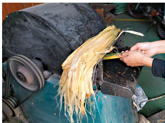
Figure 4: Fibre extraction process using decorticator
