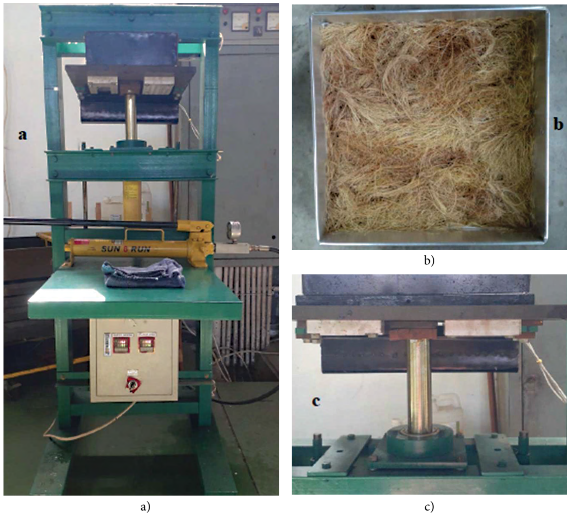
Figure 5: a) Hot press machine, b) preparation of Alpinia purpurata fibre and PLA powder in baking tray, c) pressing process
