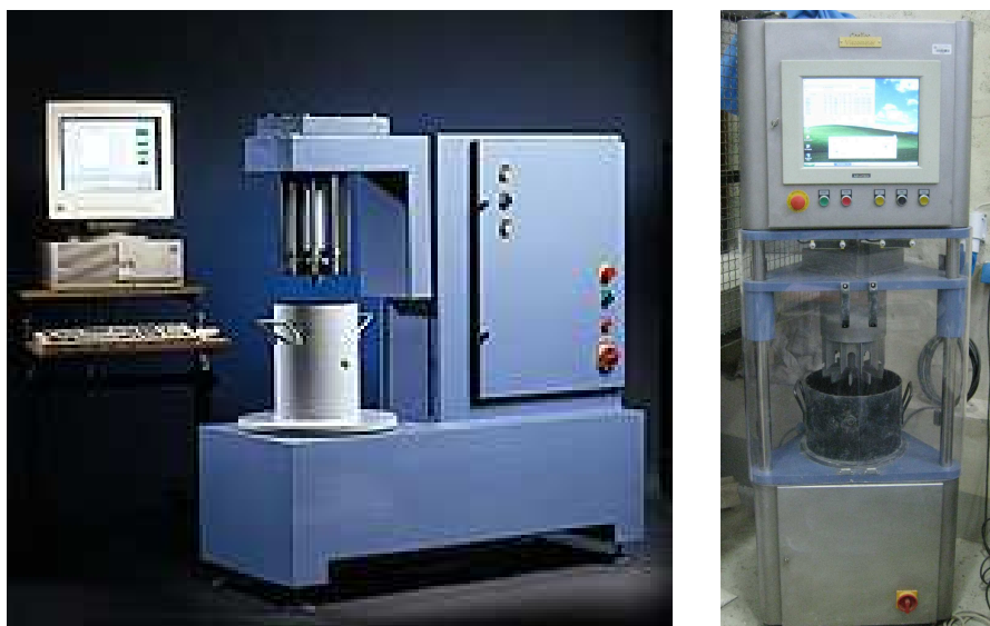
Slika 7: BML Viscometer 3 (levo) (Bartos et al., 2002; Ferraris in Brower, 2001, 2004; Koehler in Fowler, 2003) in ConTec Viscometer 5 (desno).
