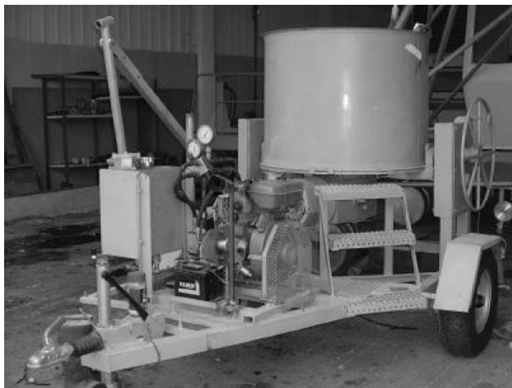
Slika 8: CEMAGREF – IMG reometer (Bartos et al., 2002; Ferraris in Brower, 2001, 2004; Koehler in Fowler, 2003).
