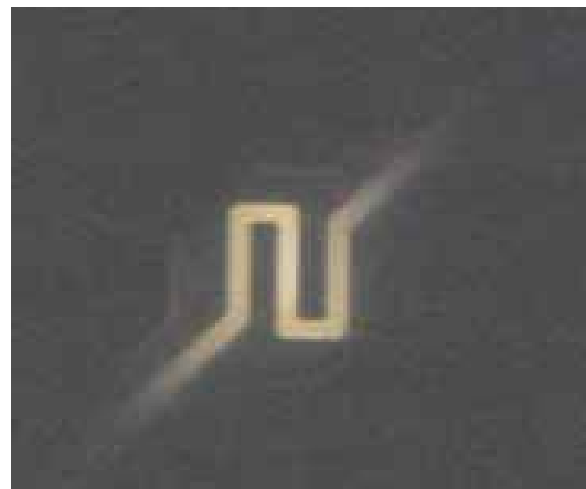
Fig. 7(b): Optical microscopy image of a glowing Pt heater on PS micro-hotplate, under 50mW power supply.
