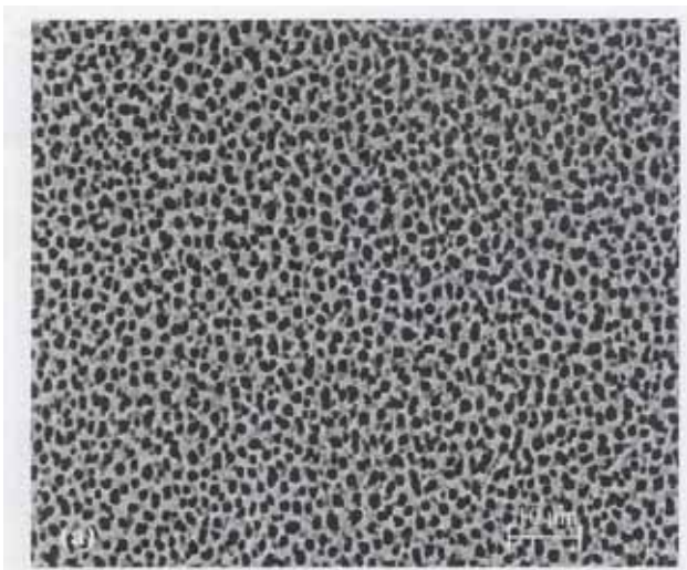
Fig. 11: (a) Plan view and (b) cross-sectional SEM images of macroporous silicon layers on bulk silicon
