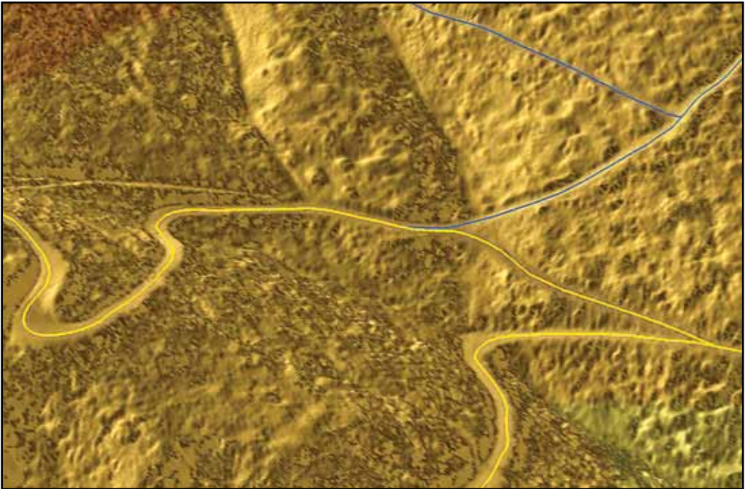
Slika 2: 3D digitalni model reliefa z jasno vidnim potekom gozdne ceste (rumena črta) in gozdne vlake (modra črta) Figure 2: 3D digital model of the relief with clearly visible course of forest road (yellow line) and forest skidding trail (blue line)
