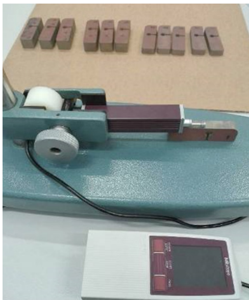
Fig. 4. Measuring equipment for the roughness
