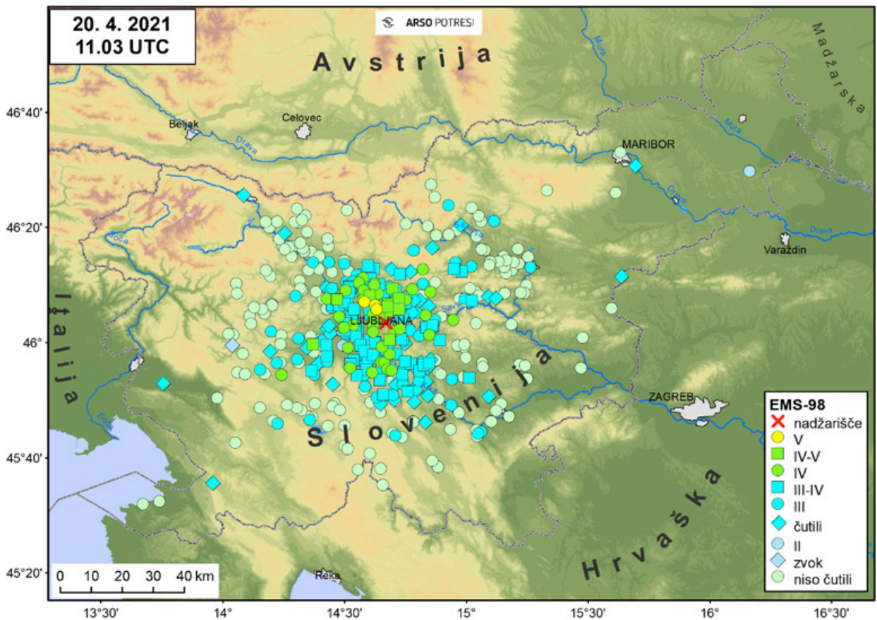
Slika 8: Intenziteta potresa magnitude 3,0 pri Klečah pri Dolu 20. aprila 2021 ob 11.03 UTC v posameznih naseljih Figure 8: Intensity of the earthquake near Kleče pri Dolu ( M_{LV}=3.0 ) on 20 April 2021 at 11:03 UTC in individual settlements. Nadžarišče = epicentre; čutili = felt; niso čutili = not felt
