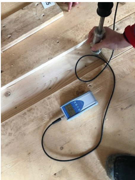
Figure 3 and 4: Monitoring with pin -type moisture meter
