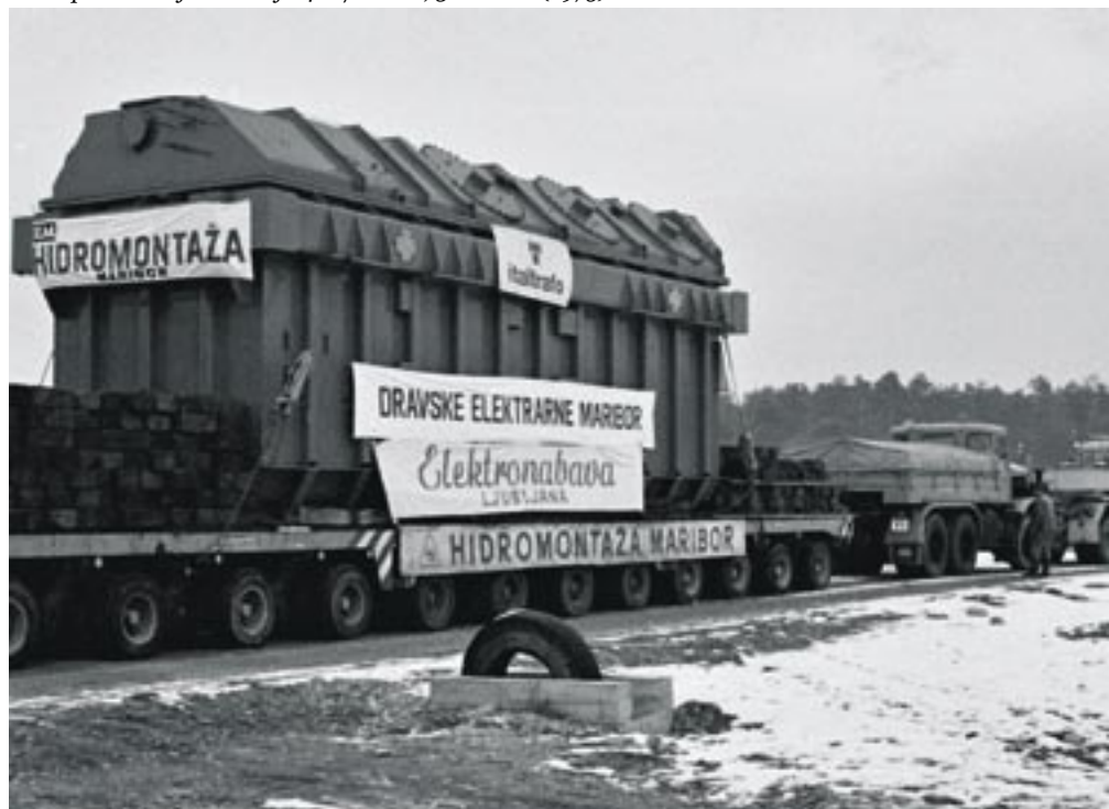
Transport transformatorja 400/110 kV, 300 MVA (1975).
