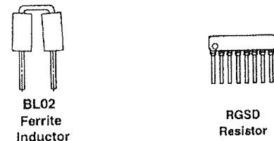
(b) Example of typical components
