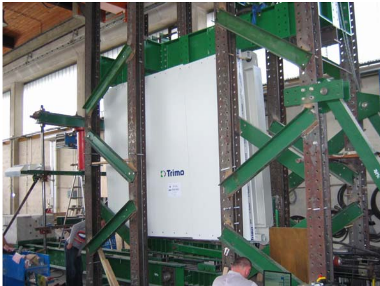
Slika B.33: Test V/2, omejen zdrs med posameznimi paneli (enostransko šivan spoj) Figure B.33: Test V/2, limited slide between sandwich panels (one-side seam connection)
