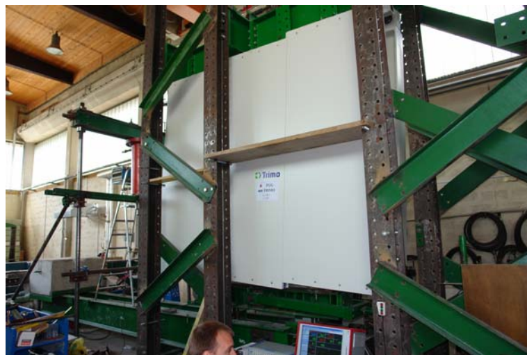
Slika B.5: Test II/1, zdrs med posameznimi paneli Figure B.5: Test II/1, slide between sandwich panels
