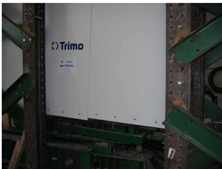
Slika B.29: Test V/1, omejen zdrs med posameznimi paneli (enostransko šivan spoj) Figure B.29: Test V/1, limited slide between sandwich panels
