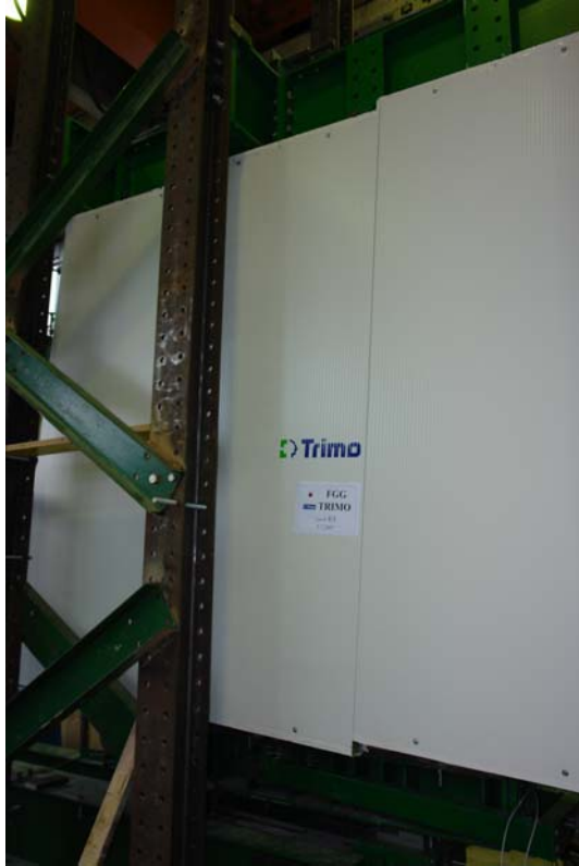
Slika B.2: Test I/1, zdrs med posameznimi paneli Figure B.2: Test I/1, slide between sandwich panels
