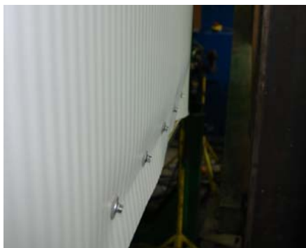
Slika 2.34: Izbočenje pločevine na zunanji strani panela pri testih III in IV serije (obojestransko šivan spoj) Figure 2.34: Buckling of the outer sheeting of the 3 rd and 4 th series of the tests
