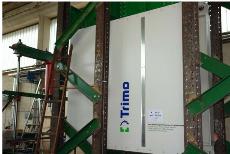
Slika B.15: Test III/2, brez zdrsa med posameznimi paneli Figure B.15: Test III/2, without slide between sandwich panels
