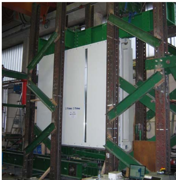
Slika 2.23: Preizkušanec III/1 s šivanim spojem in s štirimi vijaki med posameznim panelom in lego Figure 2.23: The specimen III/1 with seam connections and four bolts per meter
