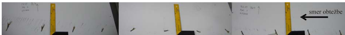
Slika 2.39: Deformiranje spodnjega roba pločevine treh panelov pri testu III-1 Figure 2.39: Deformation of the bottom side of the inner panels sheeting (test III/1)
