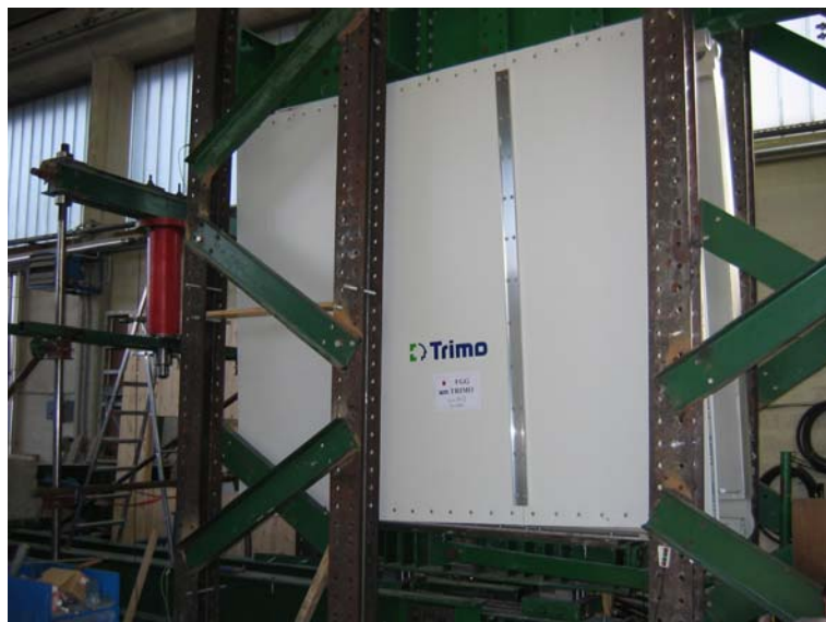
Slika B.26: Test IV/2, brez zdrsa med posameznimi paneli Figure B.26: Test IV/2, without slide between sandwich panels
