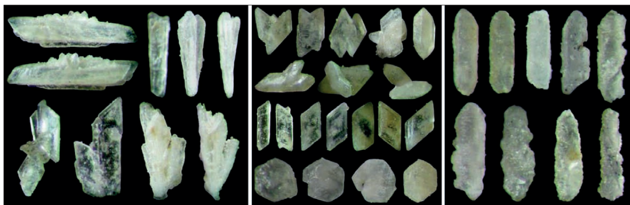
Fig. 18: Neogenic gypsum (cryogenic and usual, 0.1–1 mm in size) and celestine from the transition zone talus.
