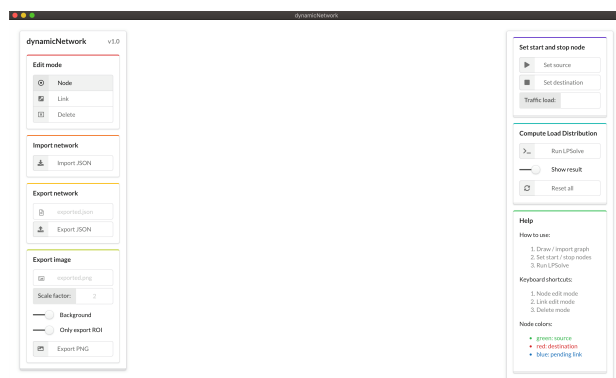
Figure 2: Grapical user interface of didactical utility, which has options for creating a new graph, exporting it in JSON format, importing an existing graph and changing the viewing options of the solution.
