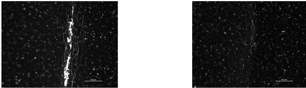
Figure 6: S5 – coating cracking when bending in MD and CD
