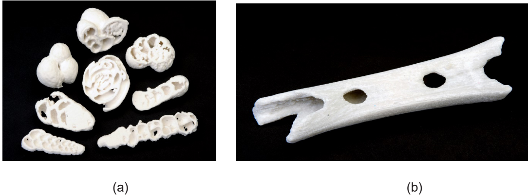
Figure 7: Items fabricated by particle-bed printing of geometry acquired by tomographic scanning shown in Fig. 4, namely (a) various foraminifera printed on an enlarged scale with exposed cross-section, and (b) a replica of the flute from the Divje babe cave.
