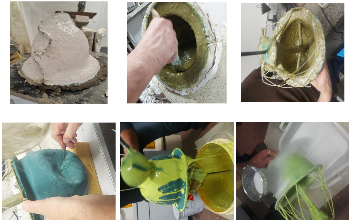
Figure 3: Silicone mould (top left), applying layers of wax to the silicone mould (top middle), constructed gating system with vents (top right), chiseling of wax (bottom left), immersion and covering of the wax model with ceramic suspension (bottom middle) and sprinkling with quartz sand (bottom right).
