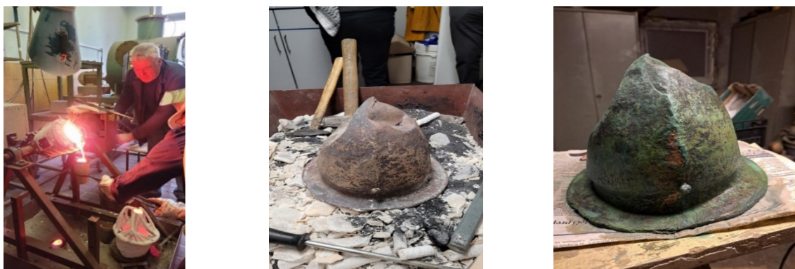
Figure 4: Pouring the leftover melt after casting the helmet (left), the helmet after casting (middle), patinated helmet (right).
