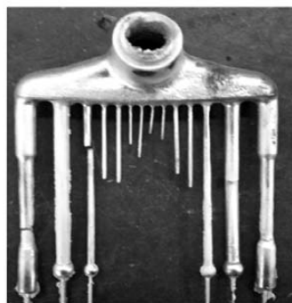
Figure 1: a) Parting plane of the metal mold for fluidity test and b) fluidity test casting
