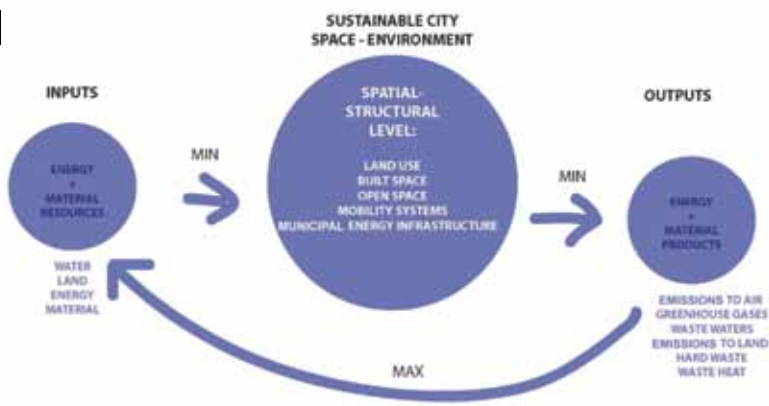
Picture 1: Scheme for sustainability principles of urban areas by the method of urban metabolism (adapted from Meijer et al., 2011)
