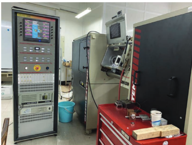
Figure 1: Gleeble-3800 thermal simulator machine
