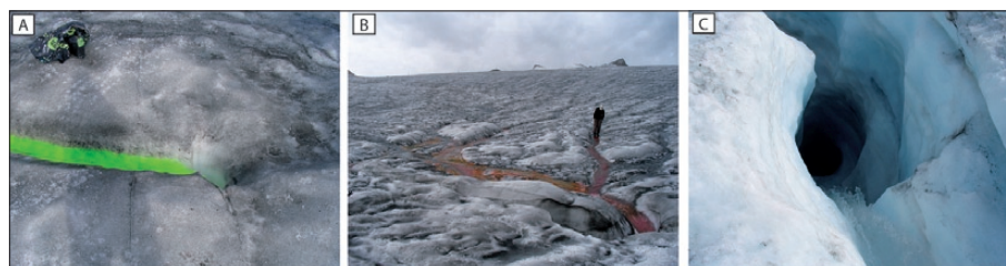
Fig. 5: Tracer injections at Tsanfleuron glacier: (A) Uranine, (B) Sulforhodamine G, (C) Naphthionate (Photos: V. Gremaud).
