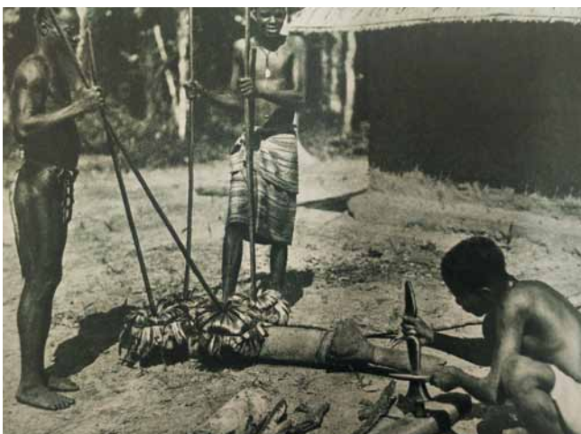
SLIKA 24: Kovač pri delu. Ob njem sta pomočnika, ki z mehom uravnata temperaturo na kurišču. FIGURE 24: A smith at work. His two assistants adjust the temperature in the forge with a bellows.
