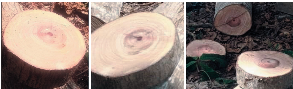
Figure 4. Samples (discs) of Terminalia catappa wood from the different parts of the tree.
