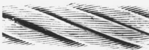
Slika 4: Jeklena vrv \varnothing 13 mm s polipropilenskim jedrom Figure 4: Wire rope \varnothing 13 mm with a polypropylene core
