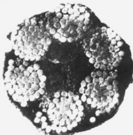
Slika 2: Jeklena vrv \varnothing 18 mm s konopljinim jedrom - prečni preiz Figure 2: Wire rope \varnothing 18 mm with a hemp core
