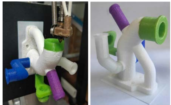
Fig. 14. Multi-branch models printed by AC-axis periodical movement (nozzle diameter: 0.4 mm)
