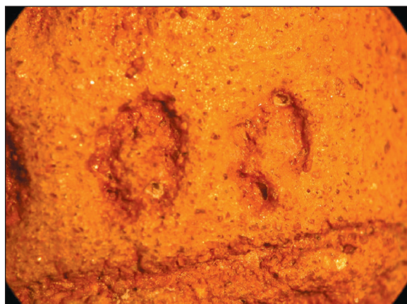
Fig. 19. The round tablet 2. Detail 1 – some calcareous areas destroyed by acid treatment.
