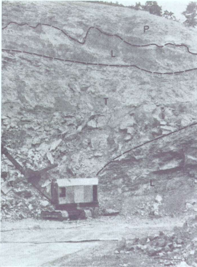
Sl. 1. Fig. 1. Kamnolom — Quarry of Gorenje. P preperel tuf — weathered tuff. L tufsko laporasti glinovec — marly tuffaceous clay. T tuf — tuff.
