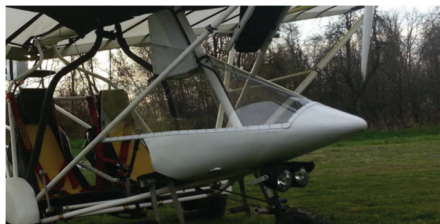
Figure 17: Installed manufactured open cabin
