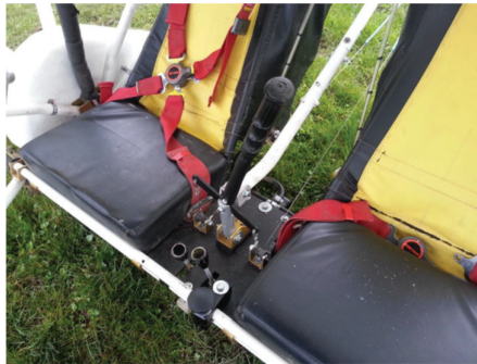
Figure 8: Modified centre stick system
