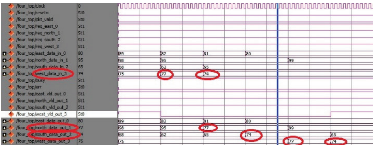
Figure7: Simulation Waveform showing the functionality of 4x4 Reconfigurable Router
