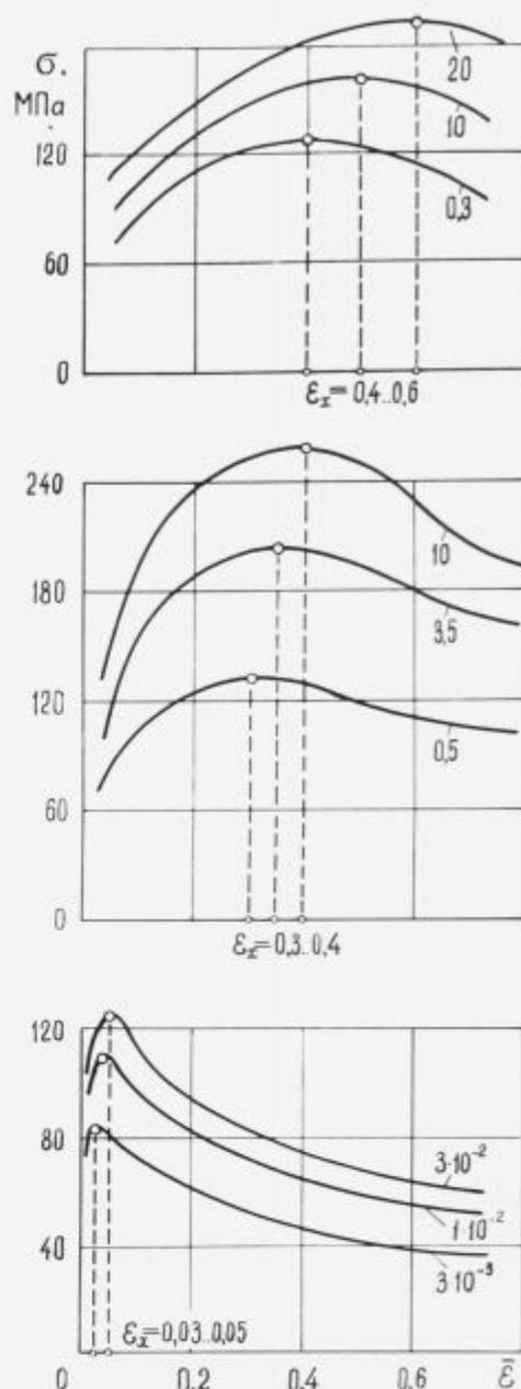
**Figure 2:** s-s curves of different rheological complexity: a - steel with 0.19% C; 0.04% Si; 0.86% Mn; 0.022% P; 0.029% S at 900°C (6); b - high speed steel with 0.88% C; 0.39% Si; 0.23% Mn; 0.03% P; 0.011% S; 3.3% Cr; 6.39% W; 4.72% Mo; 2.23% V at 1100°C (7); c - zirconium alloy with 2.5% niobium at 775°C. (8) all at the indicated values of strain rate in s<sup>-1</sup>.
