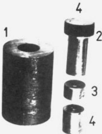
**Figure 4:** Press mould for pressing and calibration of specimens for plastometric tests: 1 - body; 2 - upper die; 3 - calibrating matrix; 4 - lower die.
