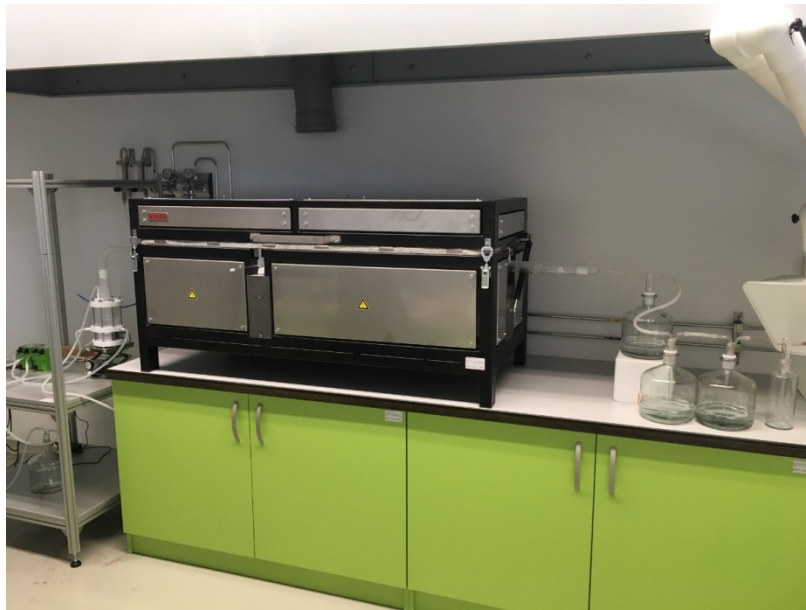
Fig. 1 Ultrasonic Spray Pyrolysis (USP) device located in Zlatarna Celje d.o.o.
