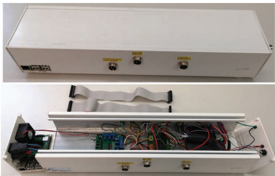
Fig. 4. Custom-made enclosure for the control hardware
