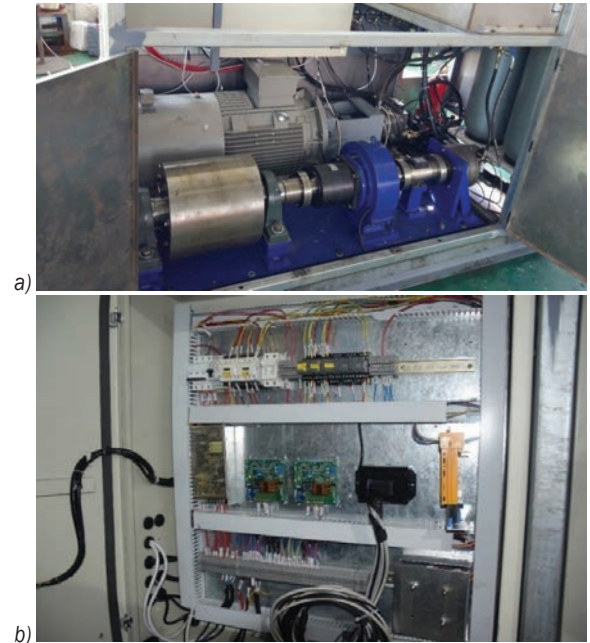
Fig. 8. Test bench; a) internal connection of test bench; and b) control panel of test bench
