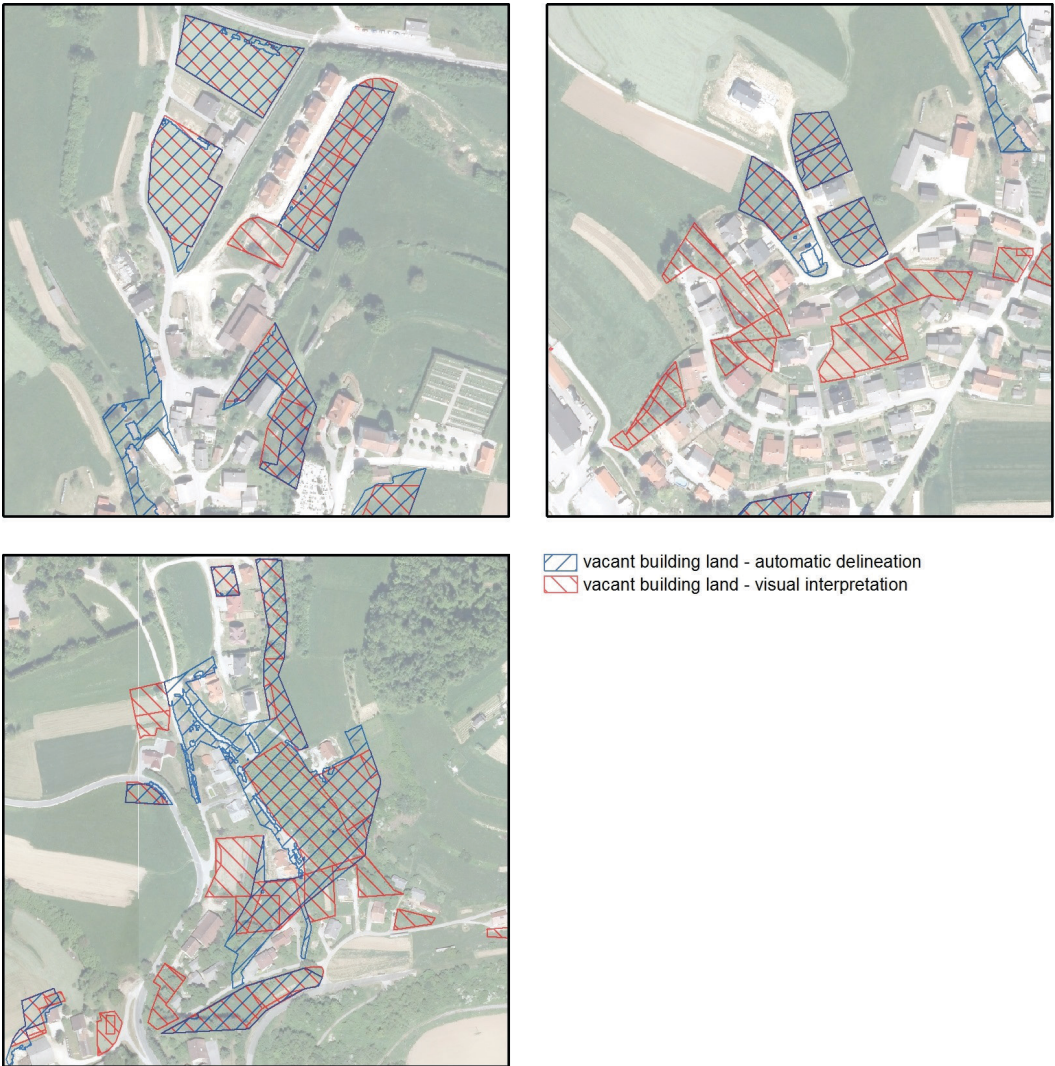
Figure 12: Detailed sections of vacant building land with the results of automatic delineation and photointerpretation – study area Veliki Gaber.
