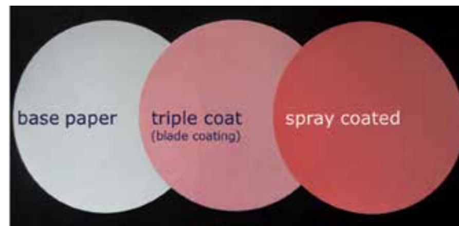
Figure 2: Laboratory cellulose-coated paper samples Slika 2: Laboratorijski vzorci premazani s celulozo
