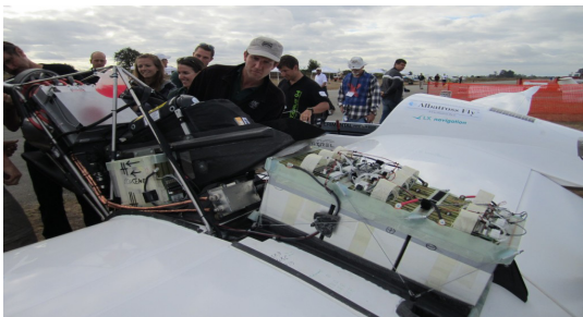
Fig. 15. Central nacelle inner elements: motor left, batteries right, parachute rescue system in the middle
