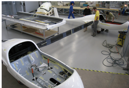
Fig. 13. Central-wing-spar fitted to wing-box assembly for the first time
