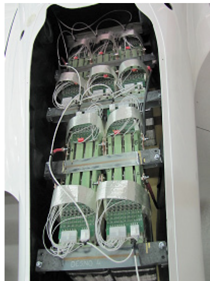
Fig.10. Battery group in one of the fuselages
