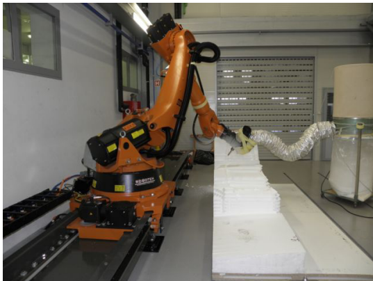
Fig. 11. Robot milling a Taurus G4 component
