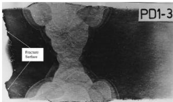
Figure 4: Macrograph of specimen PD.1-3 at a distance of 150 mm from the HAZ saw cut notch Slika 4: Makro posnetek preizkušanca PD.1-3 na razdalji 150 mm od zareze v TVP
