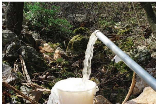
Fig. 13: Pumping test of the exploration well at the location of occasional spring Sušica (Photo: R. Biondić).
