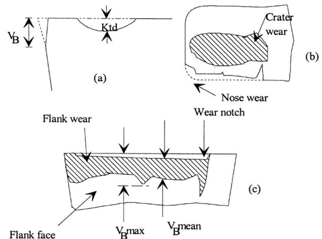
**Figure 3:** Conventional features of tool-wear measurements<sup>17</sup>
