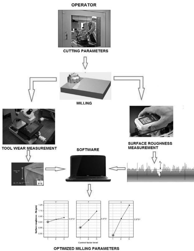
**Figure 1:** Flowchart for optimization of milling parameters
