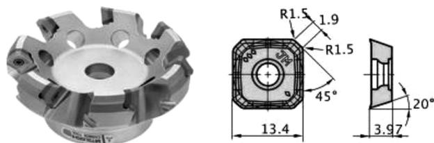
**Figure 2:** Cutting tool employed in the experiments
