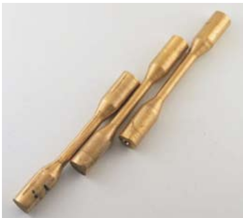
Figure 2. Tensile test tube of the dental alloy with high Au content
