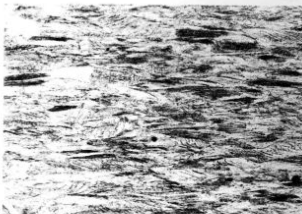
Slika 6: Mikrostruktura vlečenega stanja jekla 18/8 (povečava 100x) Figure 6: Microstructure of drawn stainless steel 18/8 (100x)
