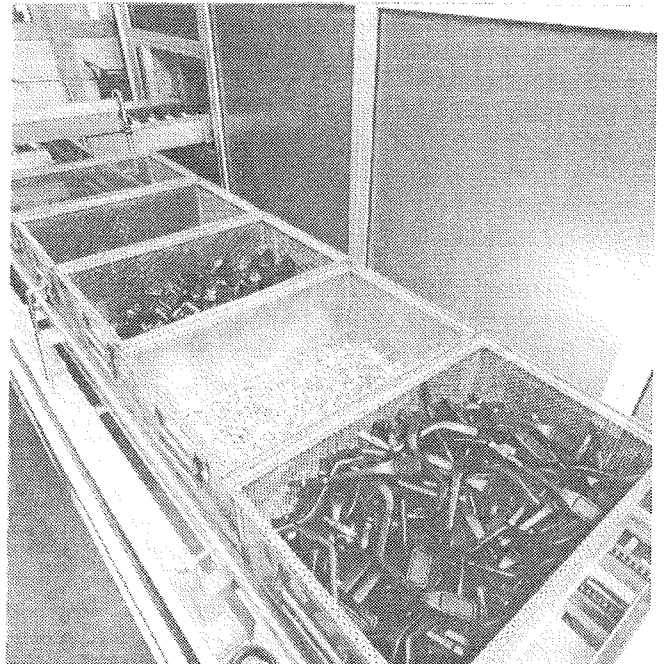
Figure 3: Combination wet/plasma cleaning of metal and plastic parts for the automotive industry
