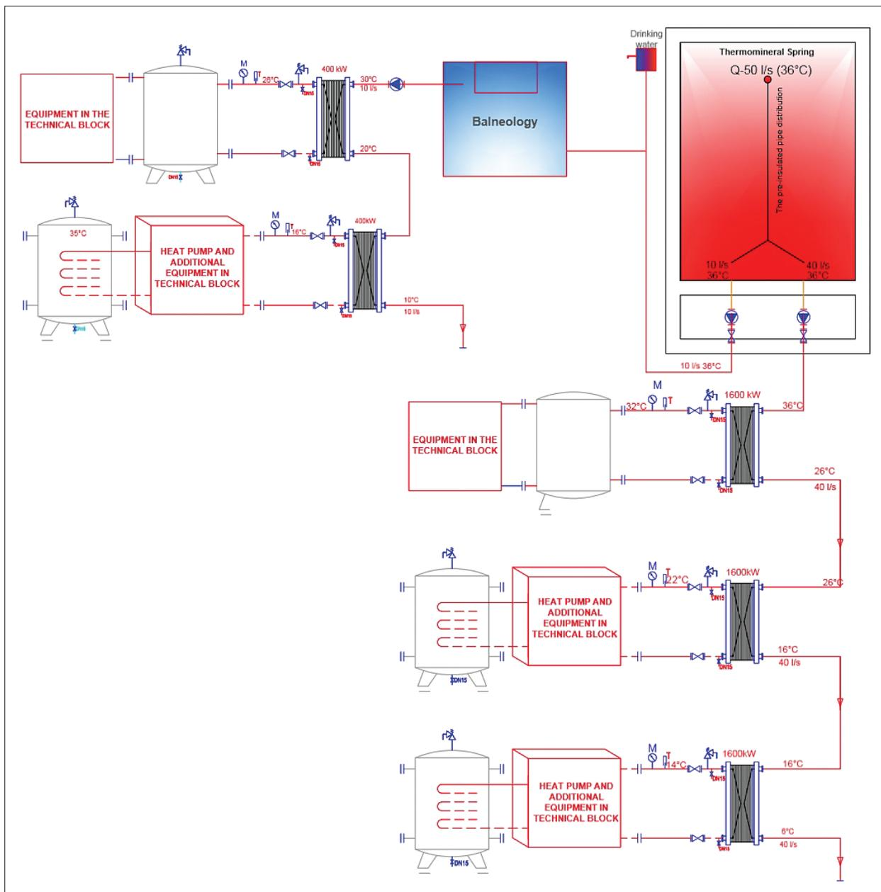
Fig. 10: Schematic survey system for multi-purpose utilisation of thermomineral waters in Pribojška Banja Spa (Milenić 2010).
