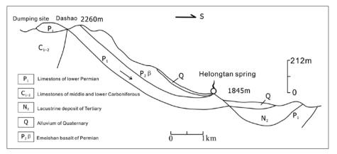
*Fig. 3: Schematic hydrogeological profile of the Heilongtan spring, north of Kunming City, Yunnan Province.*
