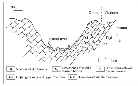
Fig. 5: Underground river polluted by manganese mining in Hurun, Guangxi.
