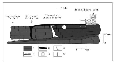
*Fig. 4: Schematic cross-section of the Laolongdong underground river in Nanshan, Chongqing,* (1) *carbonate rock; (2) sewage channel; (3) highway tunnel; (4) underground stream; (5) drinking water protection area; (6) cave sediment.*
