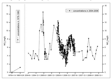
Fig. 2: Nitrate concentrations in Guancun underground river, Guangxi.
