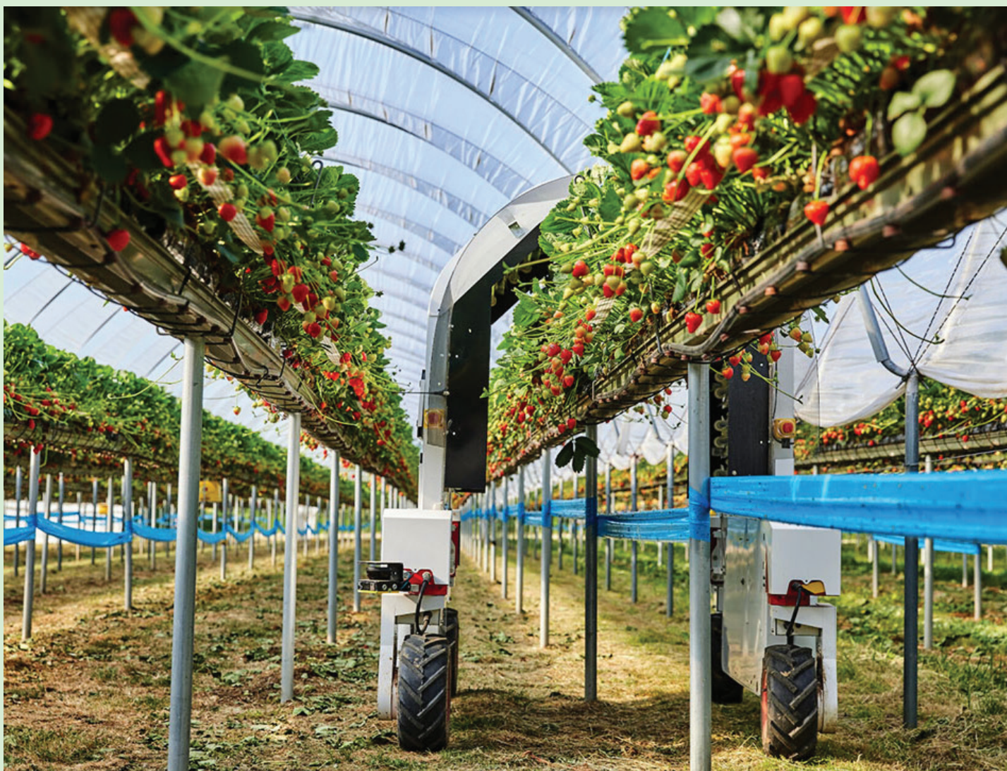
Slika 9: Mobilni robot za UV-C osvetljevanje jagod (vir: FUTURE FARMING https://www.futurefarming.com/tech-in-focus/field-robots/robot-combats-powdery-mildew-in-strawberries-using-uv-c-treatment/ )
