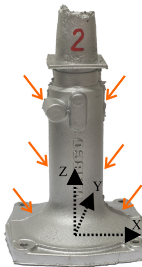
Fig. 1. Die-cast part used in the experiments. The location of the burr is indicated with orange arrows and is approximately the X-Z sectioning plane
