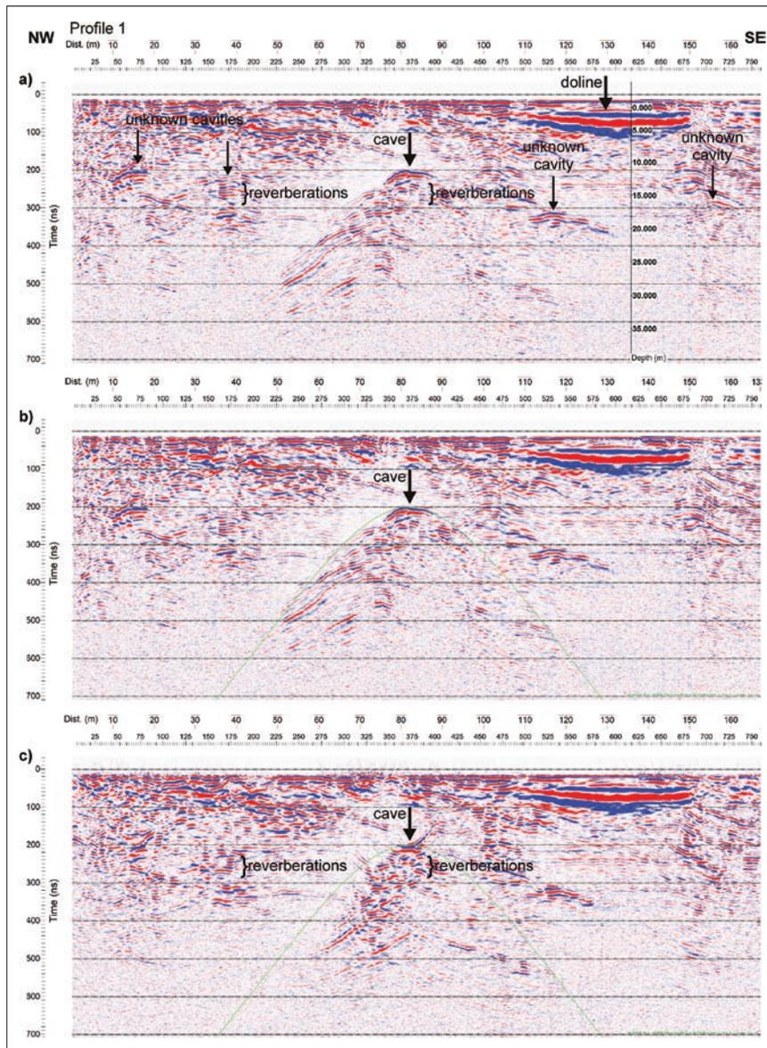
Fig. 4: GPR Profile 1 a) with time and depth scale, b) with hyperbola fitted to the diffraction caused by a cave, c) after Stolt F-K migration.
