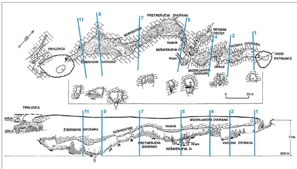
Fig. 3: Divača cave ground plan and longitudinal section with some cross sections (after Gospodarič 1985). Blue lines indicate locations of GPR profiles.
