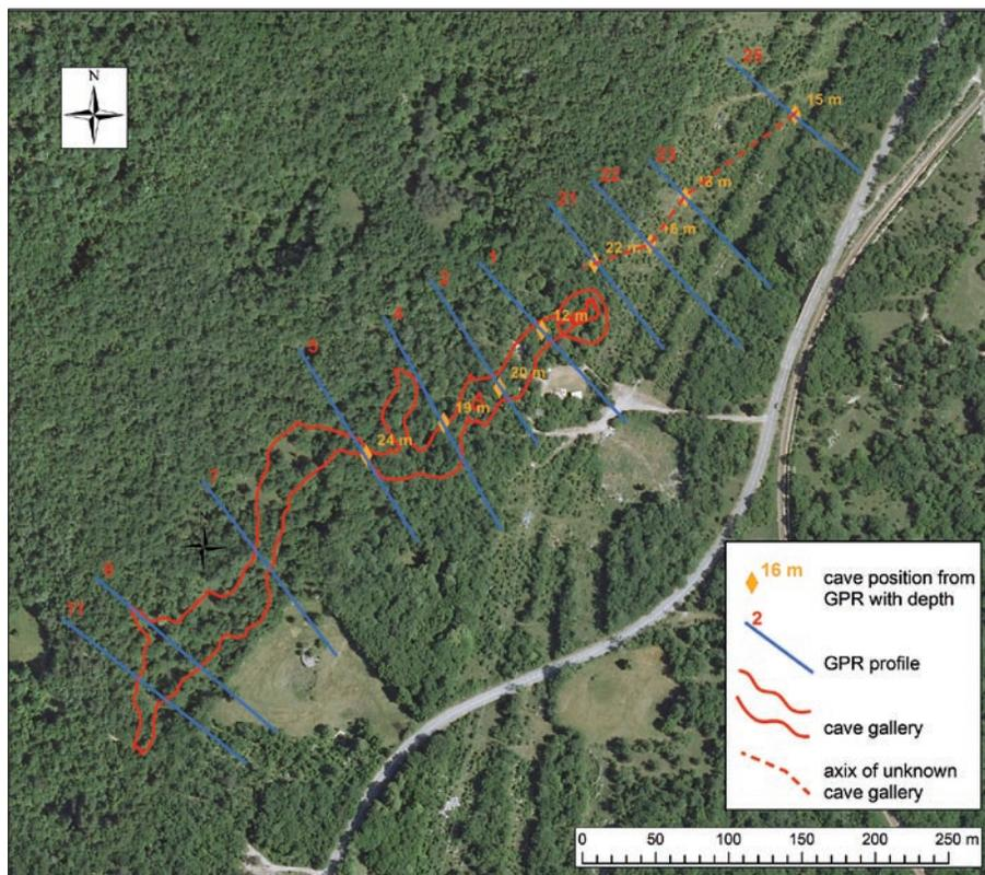
Fig. 2: Position map of GPR profiles and schematic presentation of Divača cave ground plan. Locations where the main cave gallery was revealed by GPR are indicated. Aerial image after Surveying and mapping authority of Slovenia (GURS).
