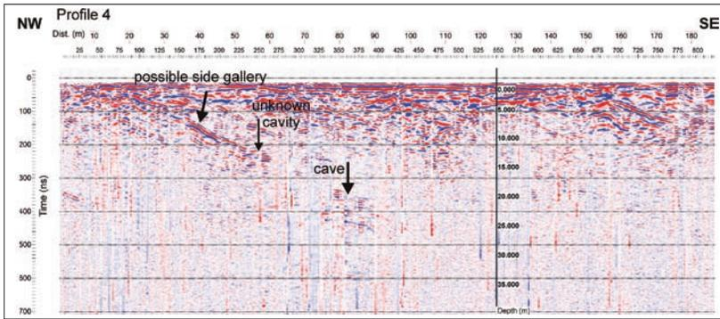
Fig. 6: GPR Profile 4 with time and depth scale.
