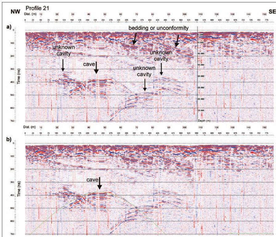
Fig. 11: GPR Profile 21 a) with time and depth scale, b) with hyperbola fitted to the diffraction caused by a cave.
