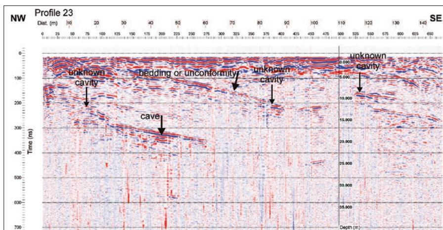
Fig. 13: GPR Profile 23 with time and depth scale.
