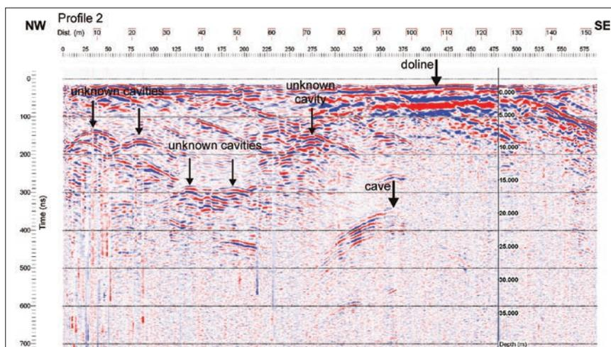
Fig. 5: GPR Profile 2 with time and depth scale.
