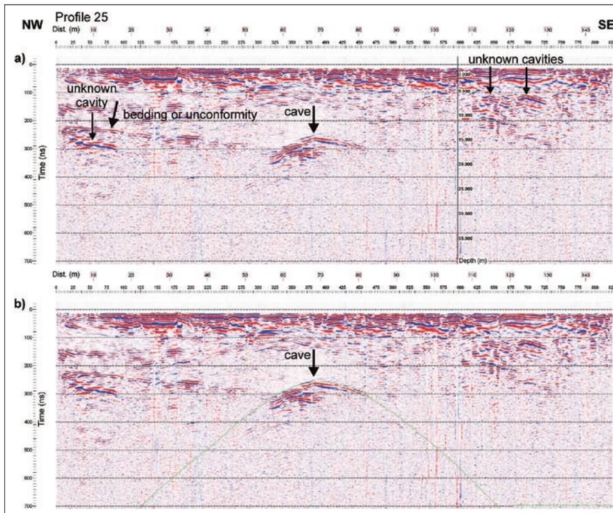
Fig. 14: GPR Profile 25 a) with time and depth scale, b) with hyperbola fitted to the diffraction caused by a cave.
