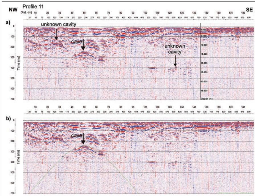
Fig. 10: GPR Profile 11 a) with time and depth scale, b) with hyperbola fitted to the diffraction caused by a cave.
