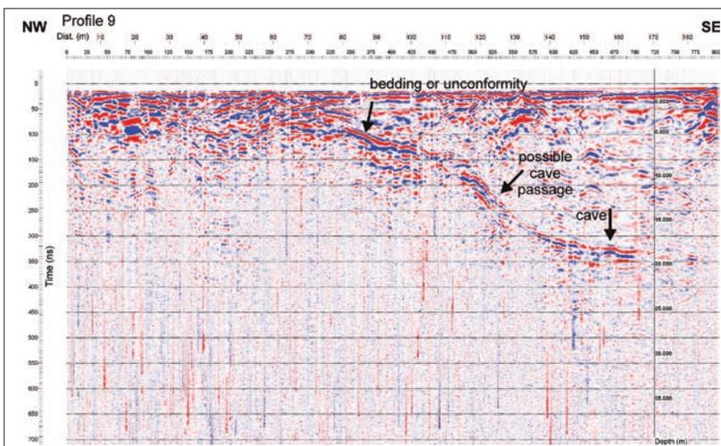
Fig. 9: GPR Profile 9 with time and depth scale.
