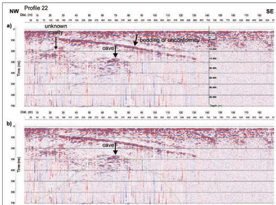
Fig. 12: GPR Profile 22. a) with time and depth scale, b) with hyperbola fitted to the diffraction caused by a cave.
