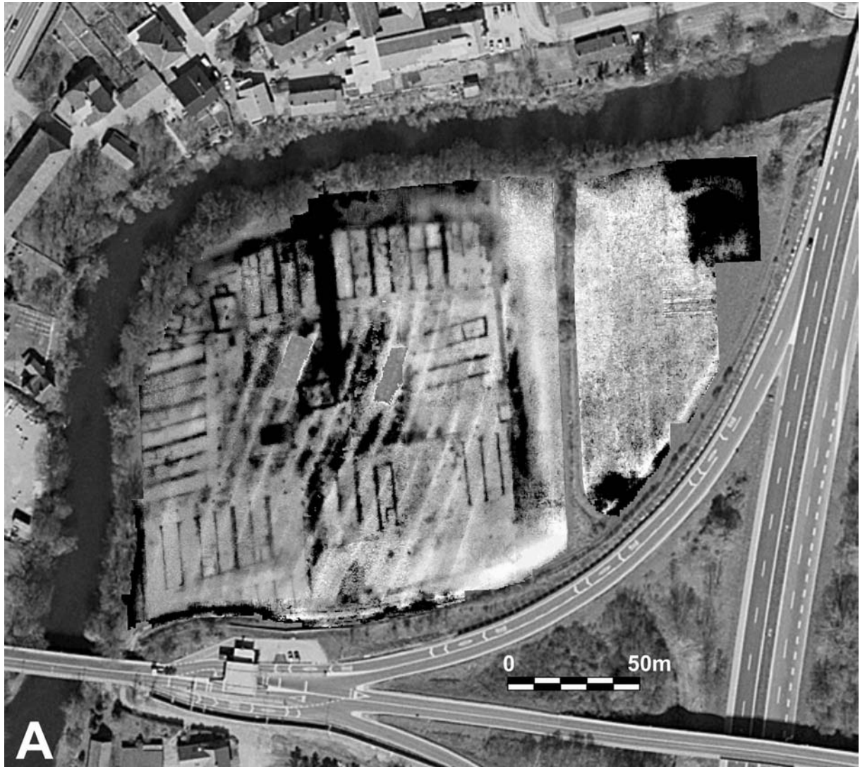
Fig. 4A: The results from geoelectric mapping on an aerial photograph. The low-pass filter with a matrix of dimensions 1 \times 1 . The span of values represents ranges between 10 and 50 \Omega . The span of values represents the range between -0.5 and +0.5 of the standard deviation (Source: © Surveying and Mapping Authority of the Republic of Slovenia, DOF at a scale of 1 : 5000 ).
