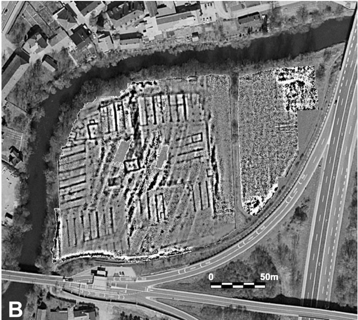
Fig. 4B: The results from geoelectric mapping on an aerial photograph. The high-pass filter with a matrix of dimensions 5 x 5. The span of values represents the range between -0.5 and +0.5 of the standard deviation (Source: © Surveying and Mapping Authority of the Republic of Slovenia, DOF at a scale of 1 : 5000).
