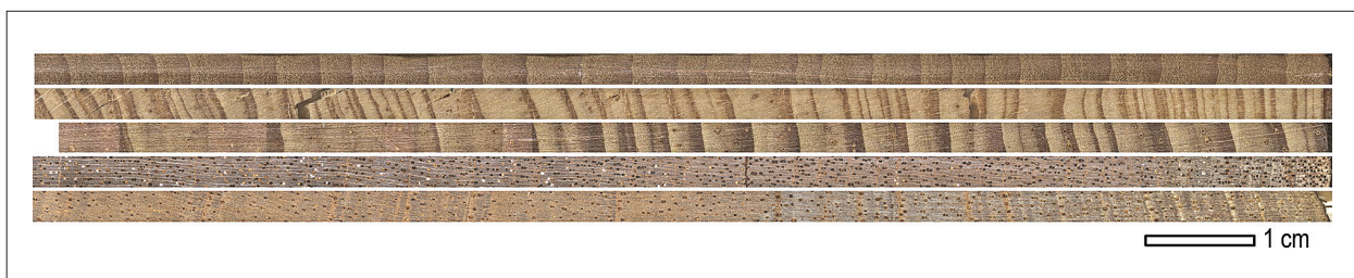
Figure 2. Stitched images of increment cores acquired with a 5x objective at the resolution of 96 dpi. From top to bottom: Fagus sylvatica , Pinus halepensis , Pinus oocarpa , Swietenia macrophylla and Cedrela odorata .
