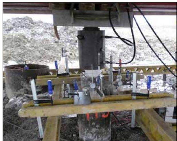
**Figure 4.** Details of the set up for the sensors in the static load test.
